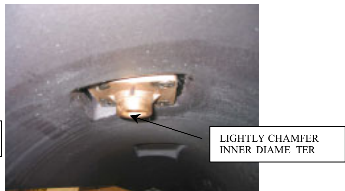
Figure 6- Inner Diameter Chamfer
